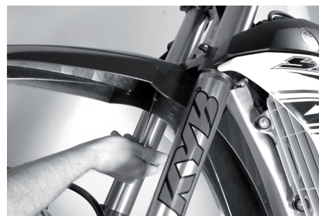
Remove the fender.
