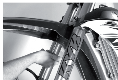
Remove the fender.
