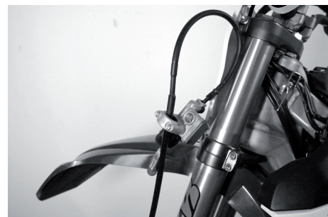
Attach the brake pump to the brake line.
