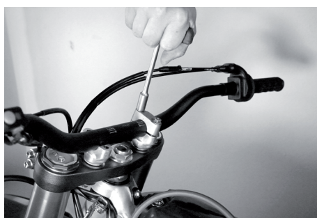
Remove the handlebar and any fastening material such as cable ties.
